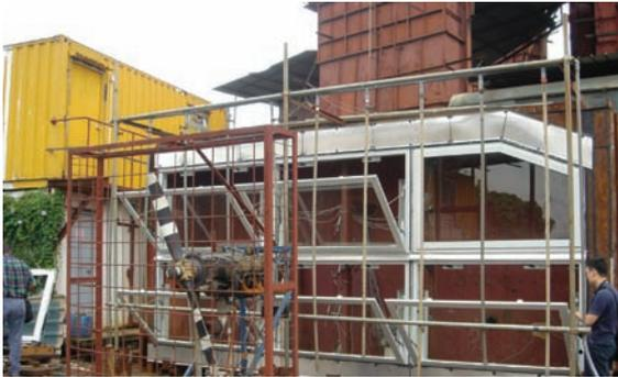
*Rain test rig for the ventilators to be installed at Sky Plaza, Hong Kong*
